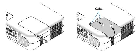
2. Loosen the two screws securing the lamp housing until the screw-driver goes into a freewheeling condition. The two screws are not removable.
